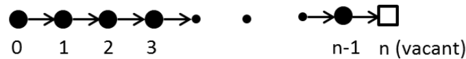
Figure 6.1 Caterpillar mechanism [117]: Cooperative jumps of n ions. All the sites from 0 to n-1 are initially filled and the caterpillar event displaces (shown by arrows) each ion by one atomic distance, or, equivalently, transfers the vacancy by n steps in the opposite direction.
